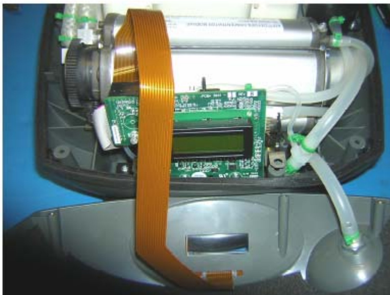
Figure 17: Membrane Panel Ribbon Cable Installation.
