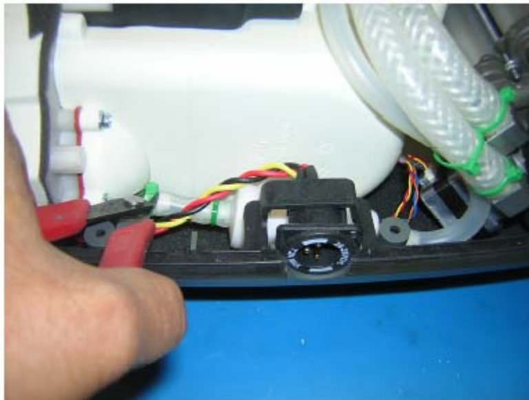
Figure 23: Removing the Compressor Intake Filter.
