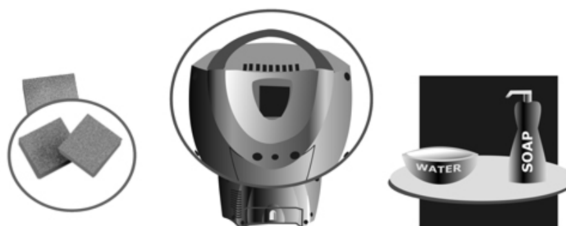
Figure 10: Cleaning the Air Inlet Filter
