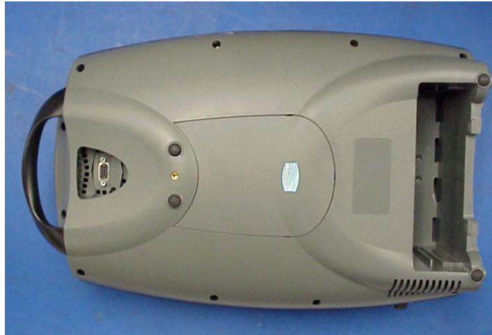
Figure 12: Removing screws to open the Front Cover
