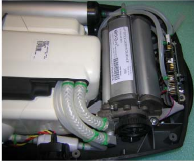
Figure 24: Installing the Compressor Intake Filter.
