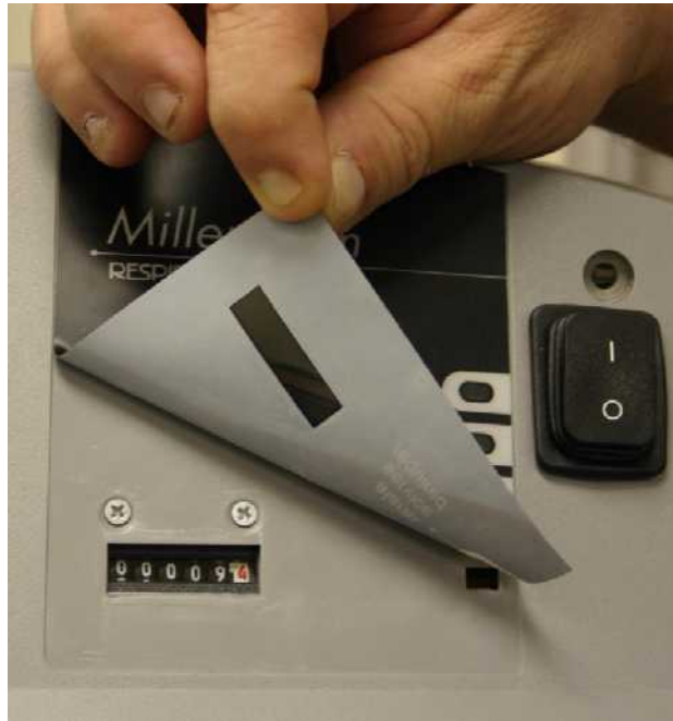
FIGURE A: REMOVING THE OVERLAY
