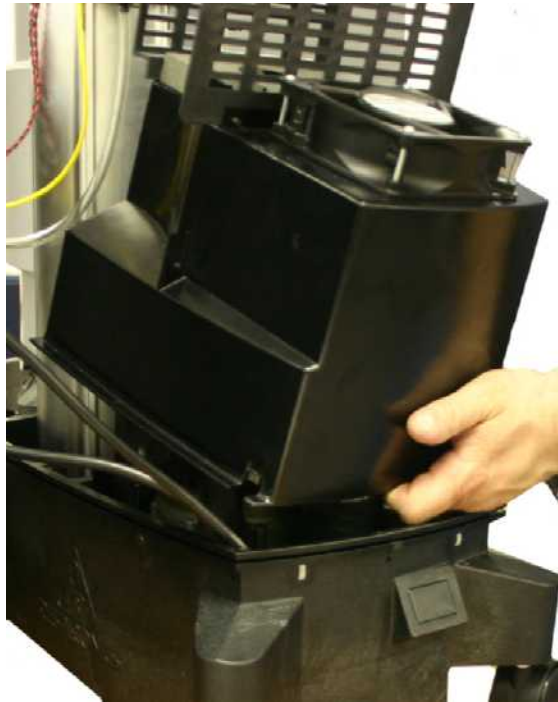
FIGURE W: REMOVAL OF THE COMPRESSOR COVER
