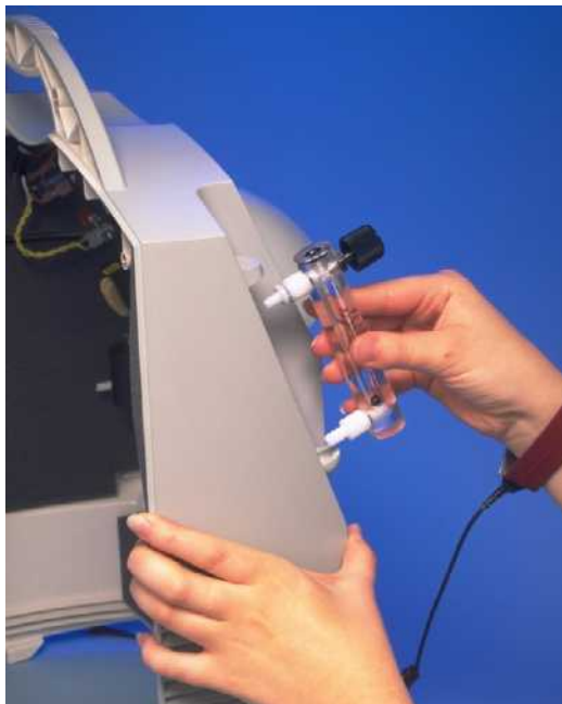
FIGURE H: REMOVING THE FLOW METER
