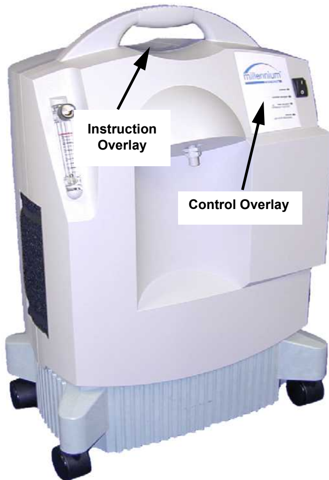
FIGURE A: OVERLAY LOCATIONS
