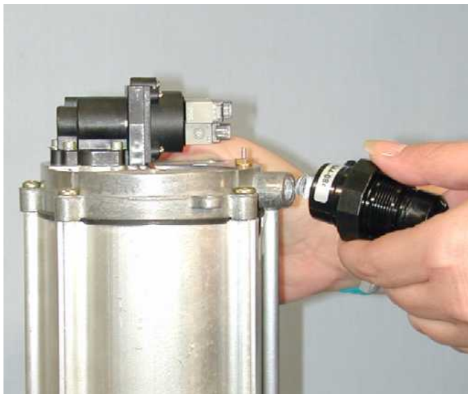
FIGURE AU: REMOVING THE PRESSURE REGULATOR
