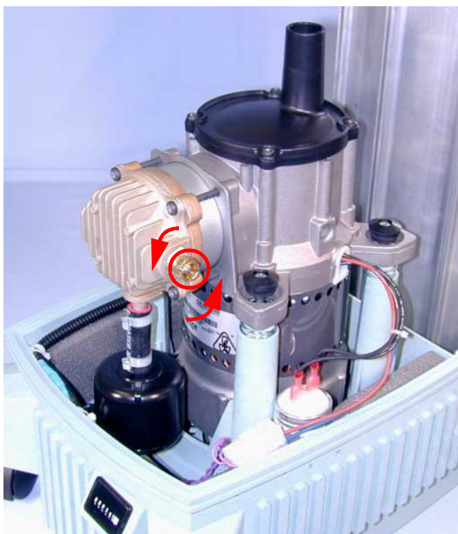
FIGURE AK: REMOVING THE PRESSURE RELIEF VALVE
