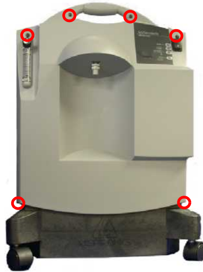
FIGURE R: SCREW LOCATIONS
