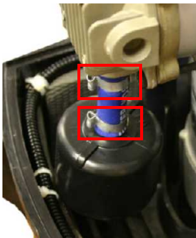
FIGURE AH: LOCATION OF THE ONE-EARED CLAMPS
