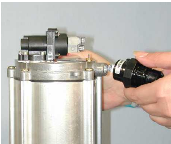
FIGURE AM: REMOVAL OF THE PRESSURE REGULATOR
