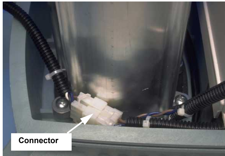
FIGURE W: LOCATION OF THE CONNECTOR
