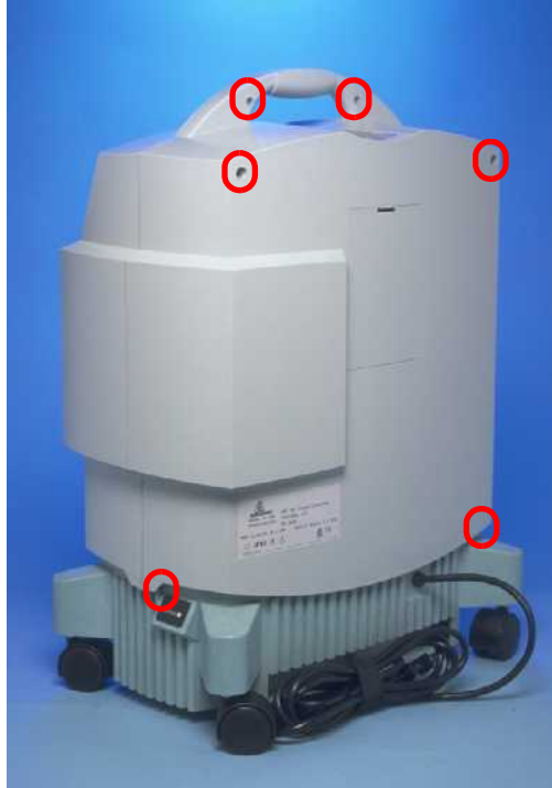
FIGURE E: REAR CABINET SCREW LOCATIONS
