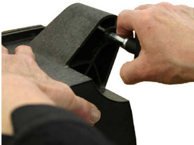
FIGURE B: CASTER REMOVAL
