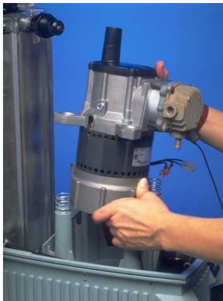
FIGURE AN: REMOVING THE COMPRESSOR ASSEMBLY
