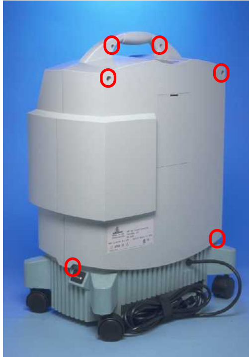
FIGURE AB: REAR CABINET SCREW LOCATIONS
