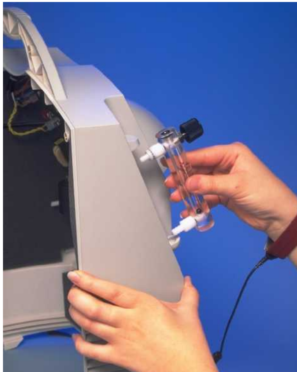
FIGURE J: REMOVING THE FLOW METER
