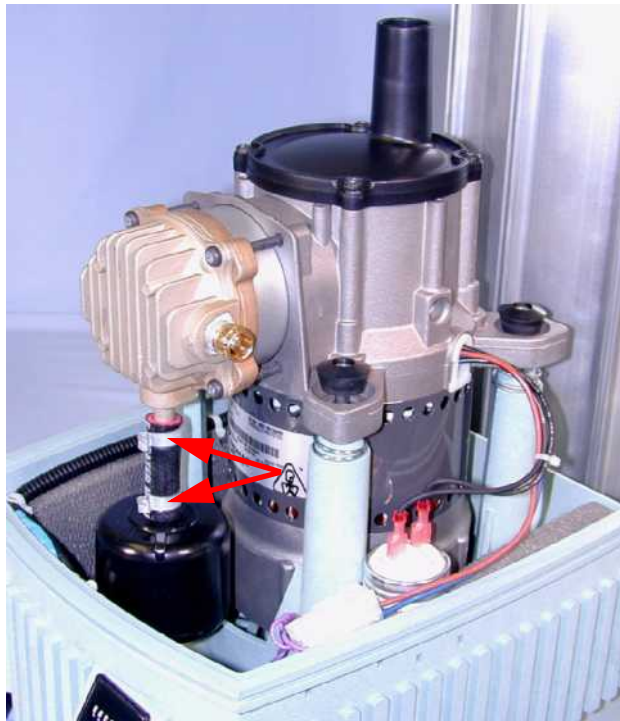
FIGURE A0: LOCATION OF THE ONE-EARED CLAMPS
