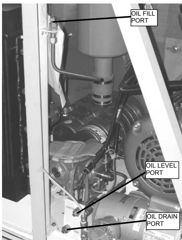
Figure 18. Blower Gear Case Oil Ports.
