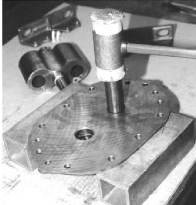
Figure 11. Tapping Bearings Out of End Plates.
