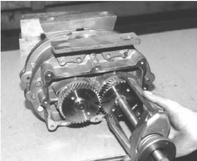
Figure 6. Pulling Drive Gear With Jaw Puller.
